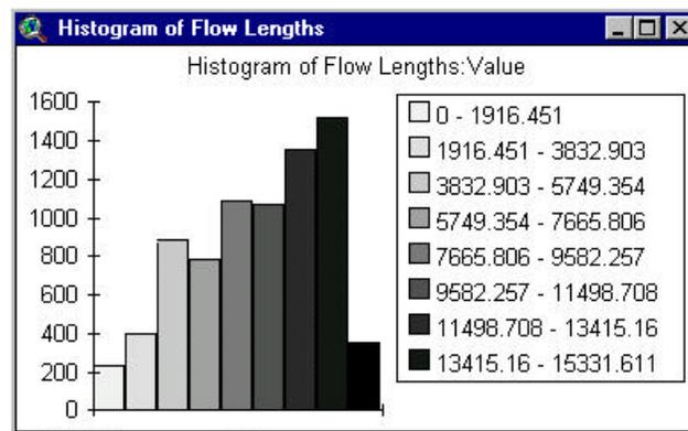
Item 3 requires some creativity to determine. You will notice that the script provided earlier uses the option “FALSE” for the “upStream” parameter. This means that flow lengths are calculated relative to the outlet (e.g. the flow length to the outlet pixel from the outlet pixel is zero). This puts the maximum flow lengths towards the extreme edges of the watershed, called the watershed divide. We can create a second grid using the opposite direction:
