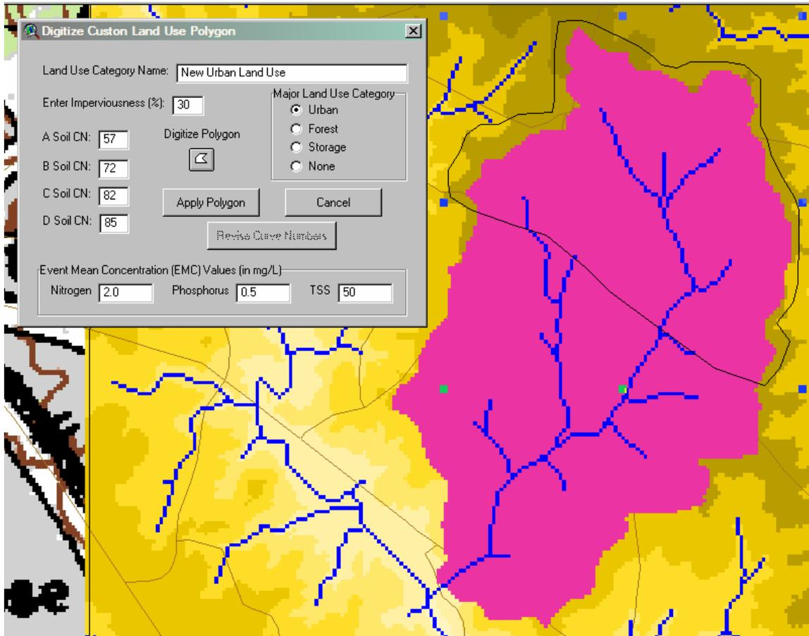
**Figure 6. Digitizing a new land use area and specifying its characteristics (imperviousness, curve numbers, and EMC values).**
